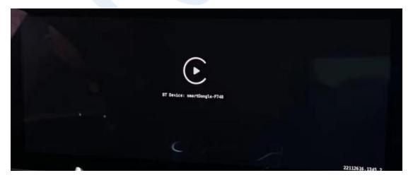
1) When we pair it for the first time, we need to keep the wifi turned on (no need to manually connect to the dongle's wifi at this time), and then perform Bluetooth pairing. When the Bluetooth pairing is successful, the wifi will automatically become connected to the dongle. You can observe whether your
